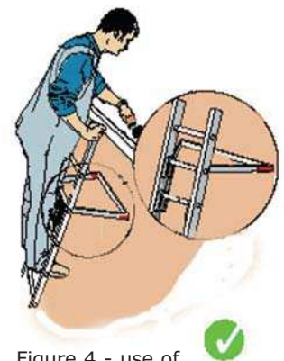
Figure 4 - use of standoff mechanism
