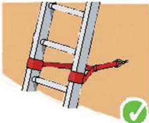
Figure 7 - Tying near the base of the ladder
