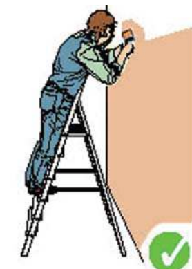
Figure 2b - keep belt buckle in the stiles
