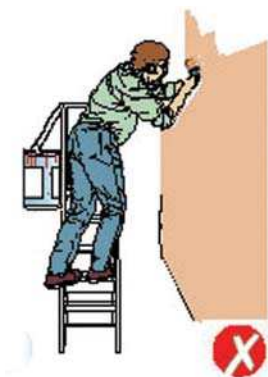
Figure 2a - avoid sideways loading
